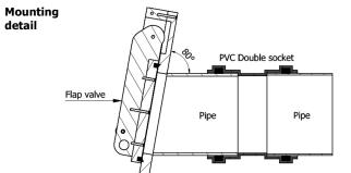
Flap valve ATKS Ø200 - HDPE/SS316L Rev.: 1 **AQUAFIX MILIEU** | Model: Spigot socket/coupling mount 10° (S) 17/7/2023 Postbus 288 3640 AG Mijdrecht T: +31 (0)297 - 26 29 29 F: +31 (0)297 - 26 12 72 Articlenr.: 670ATK0200S E: info@aquafix.nl ±6,2 kg W: www.aquafix.nl Sheet: 4 Date: 9/4/2020 Size: A3 Dwg. nr.: ATKS1900174 Des.: DG Scale: 1:7
